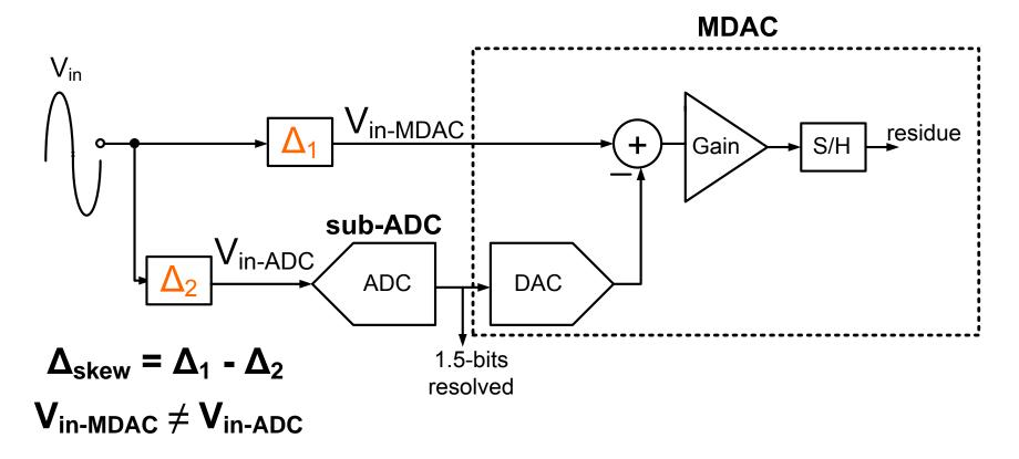
Prior works use power hungry front-end S/H to ensure MDAC, sub-ADC inputs are the same
