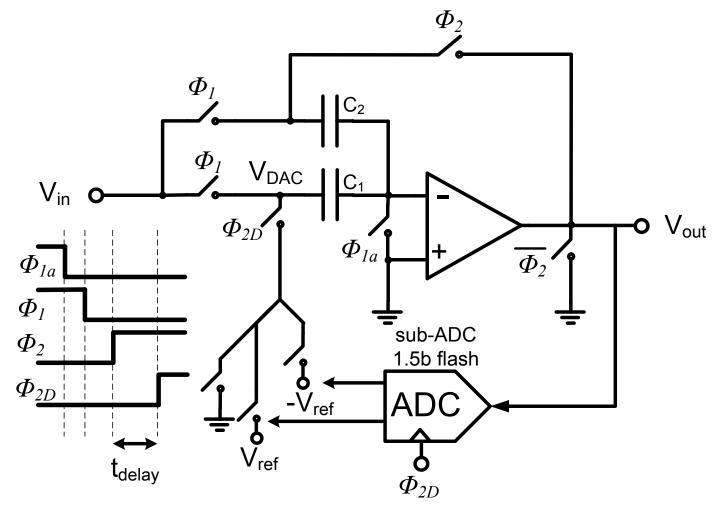
No front end Sample and Hold required to guarantee sub-ADC, MDAC operate on same input
