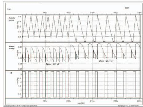
Fig. 8. Transient simulation of voltage change from 1.5 V to 2.4 at 150 mA at  $I_{LOAD} = 150$  mA.
