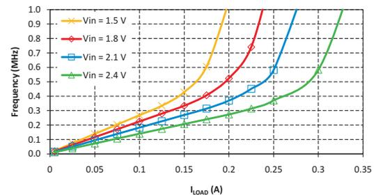
Fig. 5. Switching frequency vs. load current.
