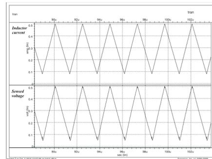
Fig. 2. Transient simulation of inductor current (top) and sensed voltage.
