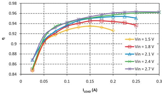
Fig. 6. Efficiency vs. load current for various input voltages.
