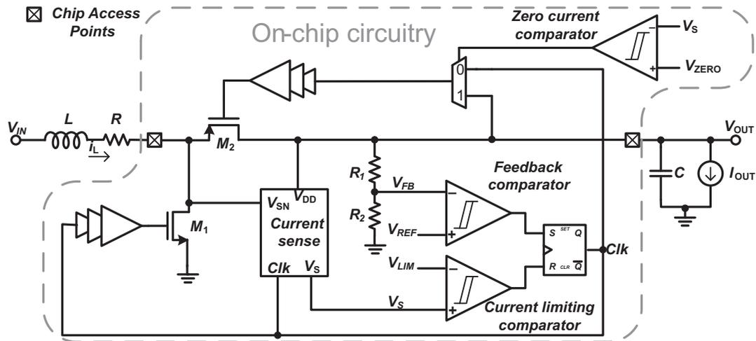
Fig. 1. System block diagram of the converter.
