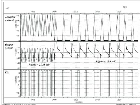
Fig. 7. Transient simulation of load change from 200 mA to 100 mA at  $V_{OUT} = 3.3$  V.
