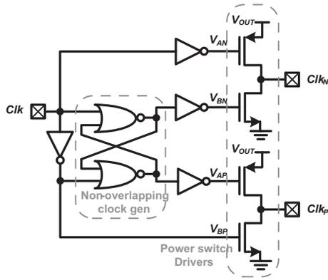
Fig. 3. Simplified diagram of power switch drivers.
