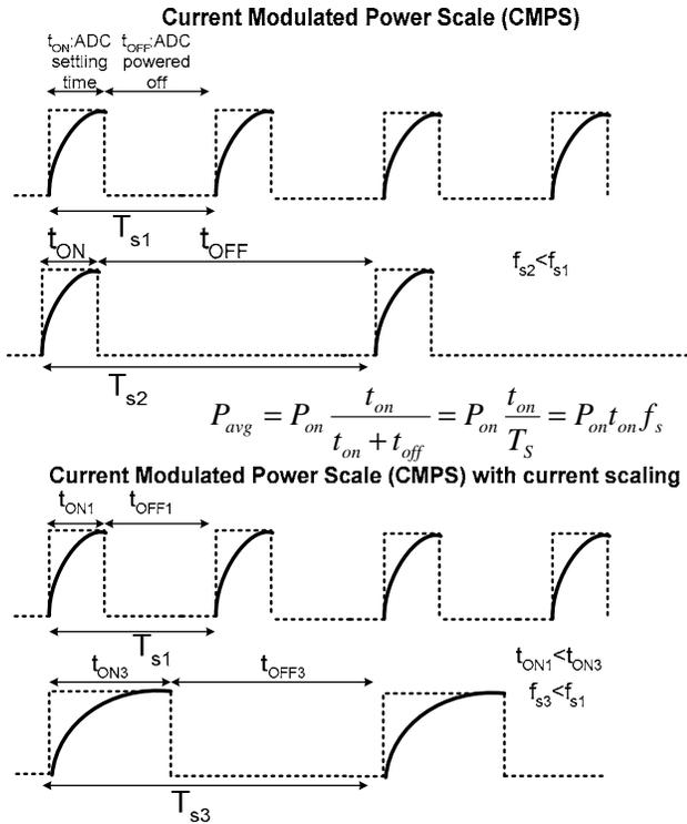
Figure 1. Current Modulated Power Scale (CMPS)
