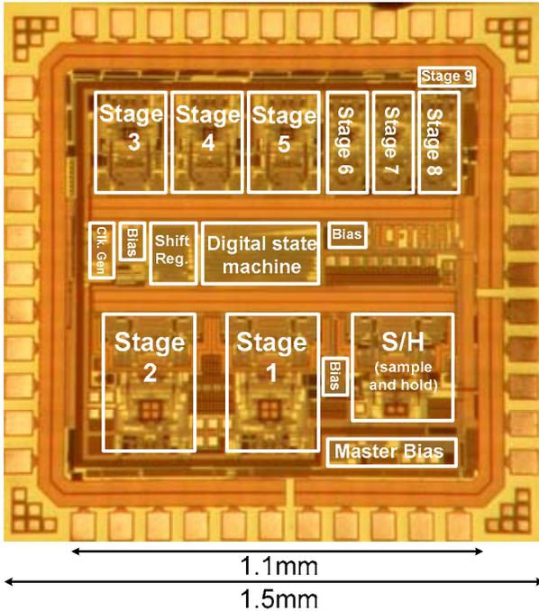
Figure 7. Fabricated ADC micrograph
