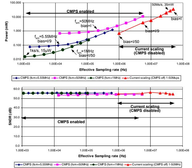
Figure 8. Power & SNDR vs.  $f_s$  for  $f_{sm}=1, 5.55, 50$ MHz
