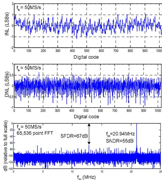
Figure 9. INL, DNL, FFT of output,  $f_s=50$ MS/s
