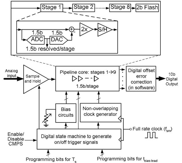
Figure 2. System Level diagram of Pipelined ADC
