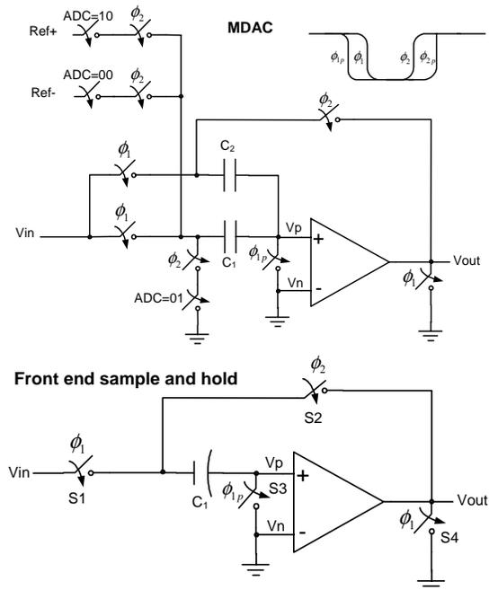
Figure 5. Stage MDAC, Front end Sample and hold
